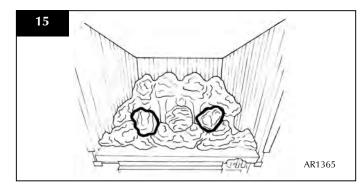
• Place another two medium size coals behind the first three coals and against the flame baffle, Diagram 16.
